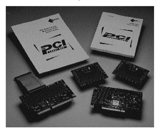
The ISA card allows the user to "emulate" an add-on processor using either the host system or a second PC. The loopback feature provides direct access to the S5933's add-on bus, enabling the user to pass commands and data through the S5933 on to the PCI bus. The uncommitted breadboard area provided by the ISA card allows for customized functionality.
